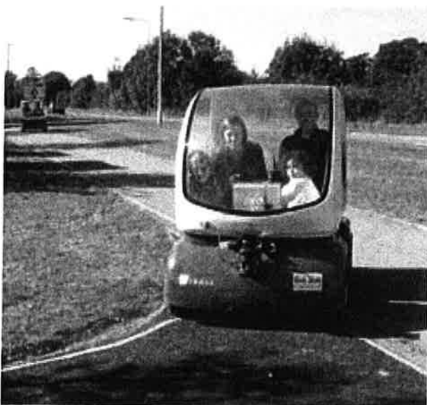
The Daventry showcase used INRIA vehicles. An operational system would run on segregated guideways.
