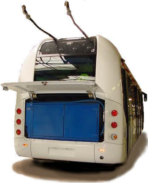
Figure 7. Group generator compartment
