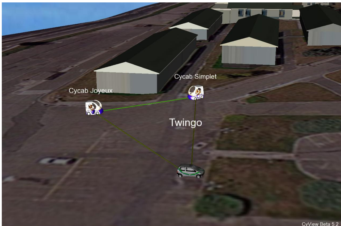
Figure 1 Management centre software showing INRIA's vehicles communication links
