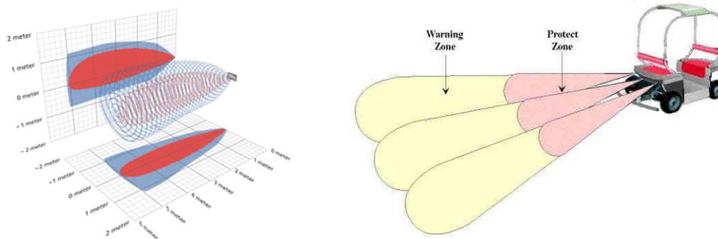
The two logical outputs of the ultrasonic module are connected to a microcontroller board. The speed modification is made by this board via the control software.
