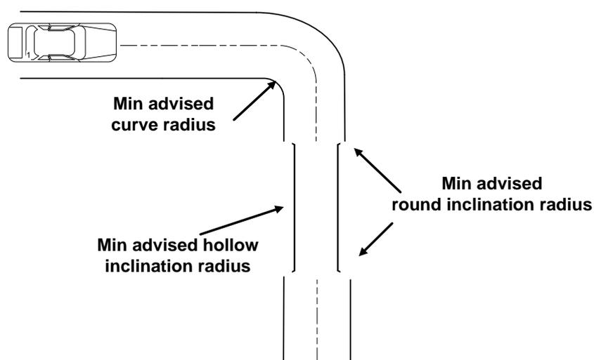
The radius of the inside curve should be the minimal advised curve radius at the defined speed for the vehicle class (car, bus, lorry etc class) at the advised minimal track width. In many countries there are guidelines that specify this radius. An example of the minimal radii for public transport in the Netherlands is given in Table 2. The inclination radius at the entrance, the top and exit of the bridge section should be set at the minimal advised value.
