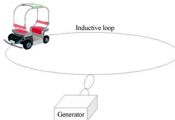
Three inductive sensors are used to follow the wire. The sensors give a voltage depending on the distance to the wire. Modifying the steering, the vehicle tries to “keep the wire” in the middle of the right and the left sensor.
